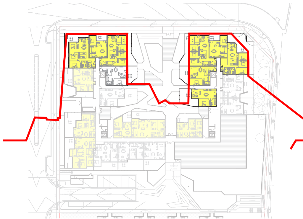
Solar Analysis - Ground Level
